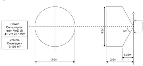
Point A relates to the installation position of the devices beacon, with the orientation such that the front of the unit faces along the X-axis of the drawing above.
