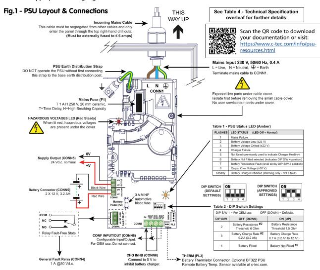
Note: On a standard 'as-supplied' unit, DIP Switch 4 is OFF (DOWN) and a fault will occur on initial power-up if fully charged batteries are NOT connected. See Table 2 - DIP Switch Settings (Fig.1).
