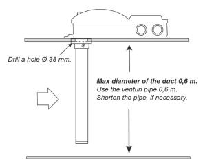
For ducts with a ø of less than 0,6 m use the 0,6 m pipe, standard. For ducts with a ø of between 0,6 m and 1,4 m use the 1,5 m pipe. For ducts which are larger than 1,4 m use the 2,8 m pipe.
