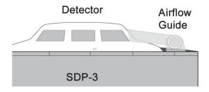
The airflow guide features a metallic airflow indicator strip which oscillates when a suitable airflow is present. If this strip isn't moving check the airflow in the duct and the mounting position of the unit.
