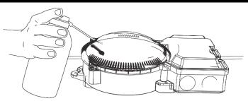
Check the airflow around the detector with a suitable smoke detector tester. Move the "test hole plug" to the side and briefly release a spray of aerosol smoke. Check the detector goes into alarm, i.e. the red alarm LEDs are activated. Also inspect the appropriate fire control panel indicators.
