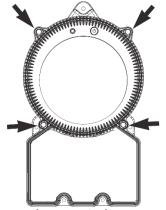
The smoke detector or sensor is mounted on a base which is fixed and wired to the SDP-3. The mounting base needs to be mounted on the centreline of the unit, using the provided fixing holes.
