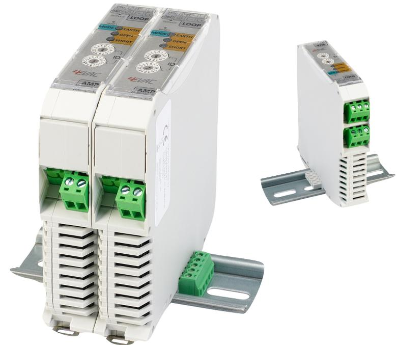
The Loop Drive Booster (LDB) is the heart of the Loopdrive system. This device drives up to 200 FIM's over a dual-core cable. A single LDB can pass 800 W of audio signal from an amplifier and injects at the same time DC to the loop for powering and managing FIM modules. One amplifier channel can be split into multiple LDB in parallel, creating multi-loop with individual surveillance for multi-zone paging applications.
