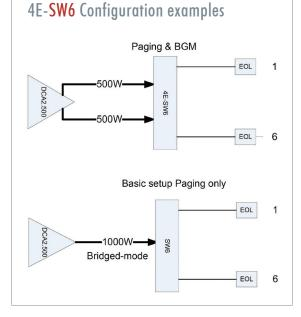
As simple and cost-effective way to distribute a variety of loads over multiple speaker-lines, small loads make a perfect match for the **4E-SW6-SWITCHING** module. Combining a single high-power 2 x channel amplifier such as the DCA 2.500 with the **4E-SW6** generates simultaneous Paging and BGM into either 6 switched speaker lines, or any multiple of 6 x channels when connected to additional **4E-SW6** modules.
