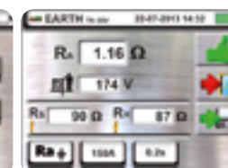
Earth resistance measurement result OK.
