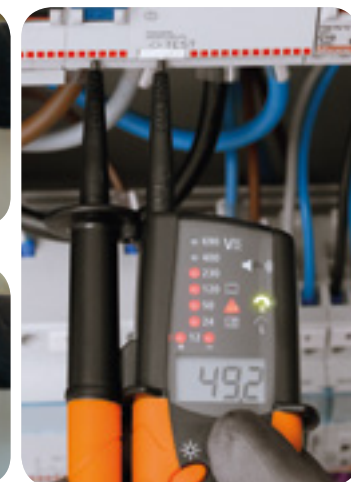
Measurement of phase sequence.
