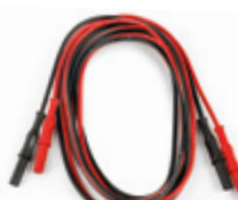
ORDER CODE HA000753 KITMPPACW SET OF CABLES GREEN - BLUE BROWN/BLACK WITH 4MM BANANA CONNECTORS Measuring range: 36A / 1000V Measurement category: CAT III 1000V Overall length: 2m Banana diameter: 4mm
