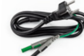
ORDER CODE HA002075 C2075 CABLE WITH BANANA GREEN - BLACK SHUKO PLUG Measuring range: 16A / 300V Measurement category: CAT III 300V Overall length: 1.5m Banana diameter: 4mm
