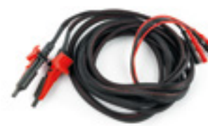
ORDER CODE HA007000 = LENGTH 3MT ORDER CODE HA700005 = LENGTH 5MT ORDER CODE HA700010 = LENGTH 10MT C7000 CABLE FOR CONTINUITY MEASUREMENT WITH CURRENT 10A OR LOOP MEASUREMENT WITH IMP57 WITH LENGTH 3M. Measurement category: CAT IV 600V / CAT III 1000V Maximum opening of alligator clip: 2.5cm Cable length: 3m Banana diameter: 4mm
