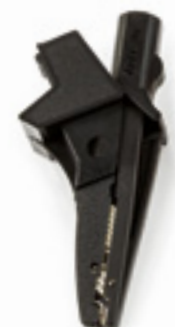
ORDER CODE HA50040# 5004-IEC# # = colour N (black) - B (blue) - R (red) - V (green) ALLIGATOR CLIP FOR CABLES WITH 4MM BANANA Measuring range: 20A / 1000V Measurement category: CAT III 1000V Maximum opening of alligator clip: 2.3cm Banana diameter: 4mm
