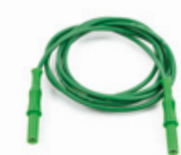
ORDER CODE HA05001# 5001-# # = colour N (black) - B (blue) R (red) - V (green) MEASURING CABLE WITH LENGTH 1.5M WITH VARIOUS COLOURS AVAILABLE Measuring range: 10A / 1000V Measurement category: CAT IV 600V / CAT III 1000V Overall length: 1.5m Banana diameter: 4mm
