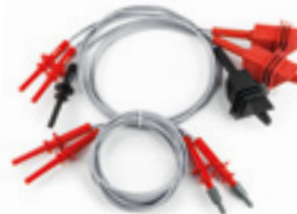
ORDER CODE HA014000 KIT14000 SET OF CABLES OR INSULATION MEASUREMENTS UP TO 5KV Measuring range: 10A / 5000VDC Measurement category: CAT IV 600VAC, CAT III 1000V, CAT I 5000VDC Maximum opening of alligator clip: 2.3cm Overall length: 2m Banana diameter: 4mm
