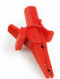
ORDER CODE HA000144 YAAMK0001HTO PAIR OF TEST LEADS ALLIGATOR CLIPS COLOUR RED/BLACK 4MM Measuring range: 10A / 1000V Measurement category: CAT IV 600V / CAT III 1000V Maximum opening of alligator clip: 3cm Banana diameter: 4mm Can only be used with YAAMK0000HTO leads
