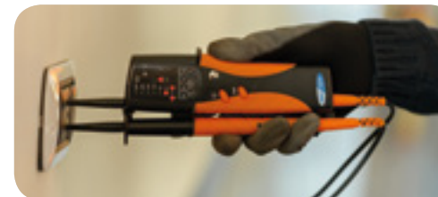
Multimeter function with display and LED indication.
