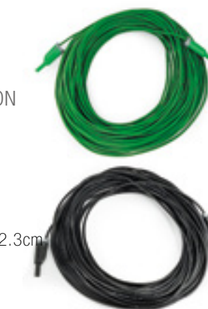
ORDER CODE HA014000 KITPVEXT25M 25M EXTENSION CABLE FOR MEASURING I-V, ISC AND VOC Measuring range: 20A / 1000V Measurement category: CAT IV 600V / CAT III 1000V Extension cable connectors: 1066-IEC# Banana diameter: 4mm
