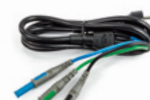
ORDER CODE HA02033X C2033X CABLE WITH BANANA GREEN - BLACK - BLUE SHUKO PLUG Measuring range: 16A / 300V Measurement category: CAT III 300V Overall length: 1.5m Banana diameter: 4mm
