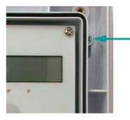
Screw in through holes provided outside of the rubber seal. Wire to head using colour coded terminals.
