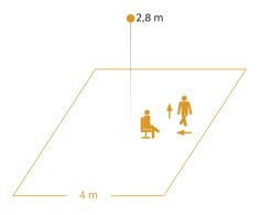
Possible mounting height: 2,50 m - 4,00 m Orange: presence, tangential and radial
