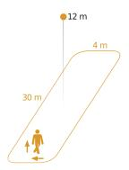
Possible mounting height: 4,00 m – 16,00 m Orange: radial and tangential
